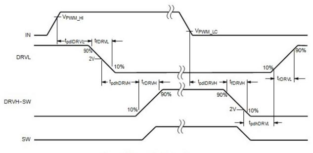
Figure 3. Nonoverlap Timing Diagram
