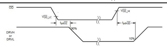
Figure 2. Output Disable Timing Diagram
